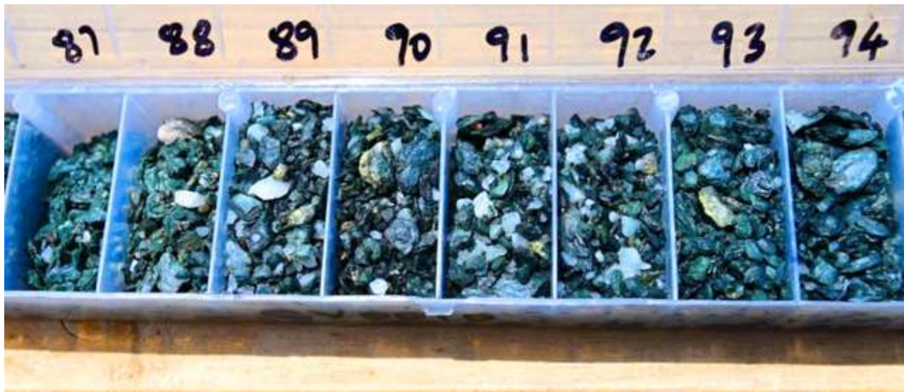
Figure 2: A small section of Copper mineralisation (chalcopyrite) intersected in RC chips from hole CV0010, 87 to 94m shown of a broader mineralised interval of 84 to 96m
